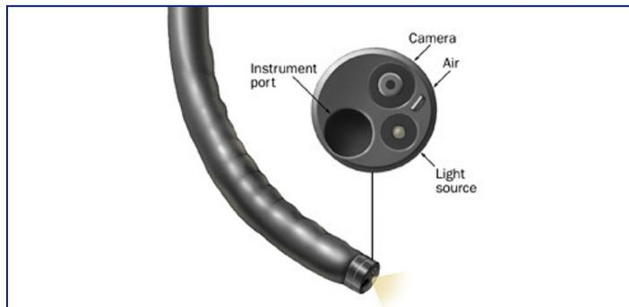
**Figure 8.** Single-channel endoscope.
