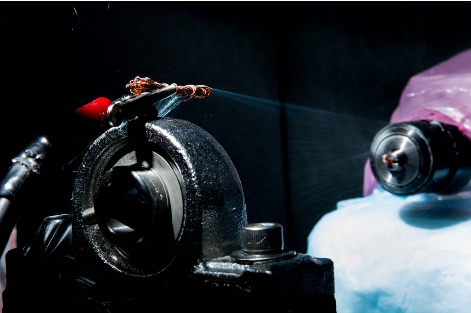
Kunal Parikh's in-house spinning system produces a multifilament suture that is capable of releasing incorporated drugs over long periods of time.
