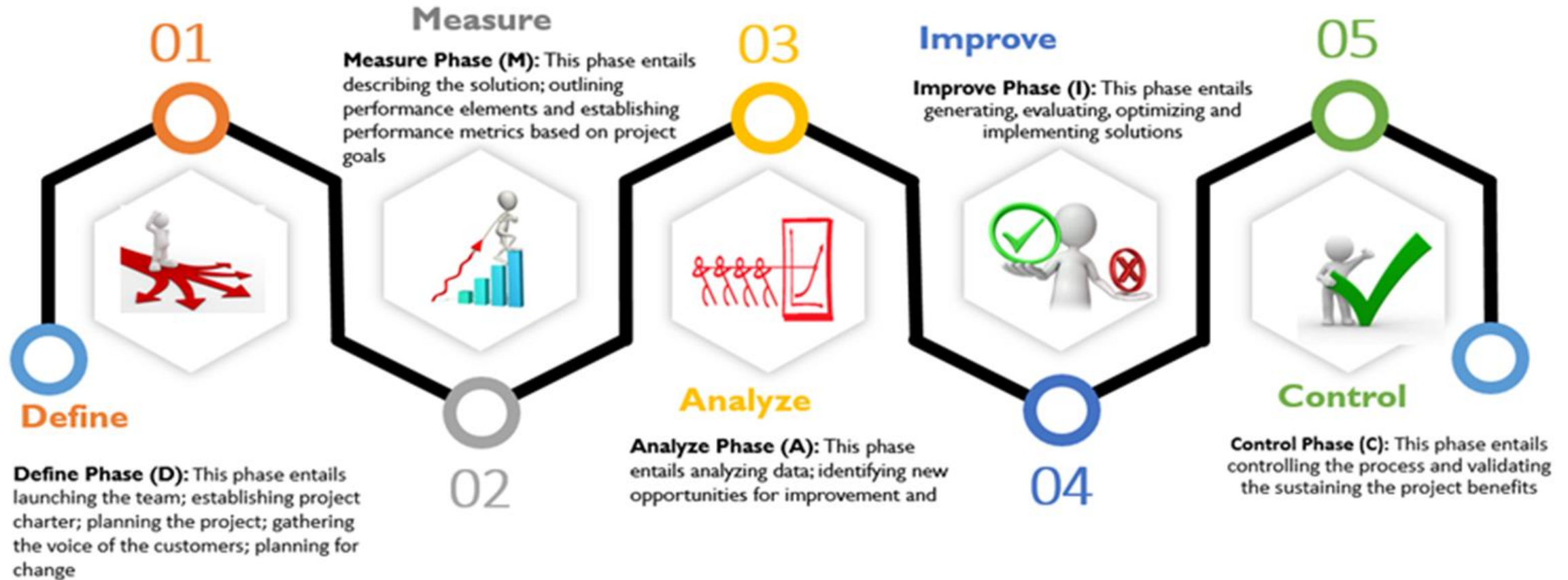
Figure 1. In developing this program we followed a Define, Measure, Analyze, Improve and Control (DMAIC) Six Sigma Methodology. This methodology is used to optimize and stabilize processes, eliminate waste, decrease variation and sustain performance improvement
