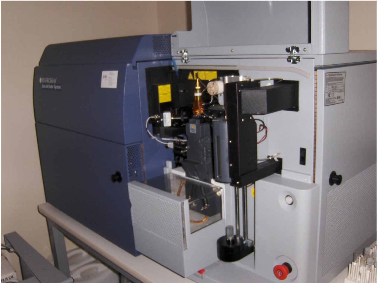
SIXTEEN PARAMETER SPECIAL ORDER SYSTEM (BD BIOSCIENCES) WITH 2 LIGHT SCATTER AND 14 FLUORESCENCE DETECTORS
